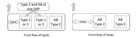
Figure 1 - Schematic of air bag (AB) and seat belt protection for vehicles without driving controls and fewer than 2 outboard DSPs (provided for illustration purposes only)
